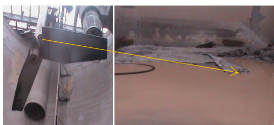
Fig. 5 Mechanical Failure of an Agitator Blade
