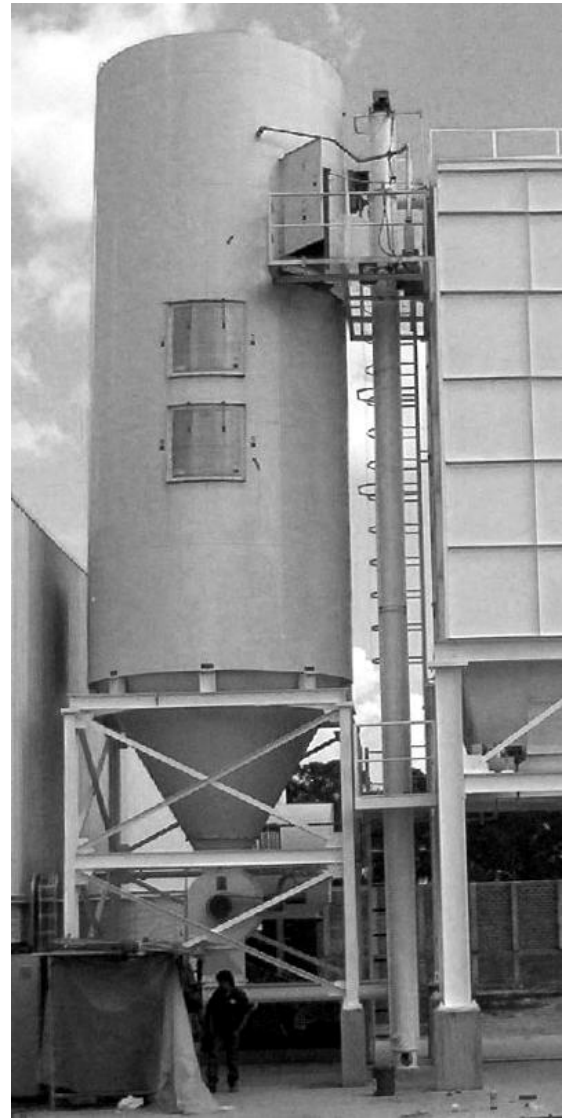
The Screw-Lift does an efficient elevating job as part of a complete Screw Conveyor system. The Screw-Lift illustrates the compact arrangement possible when space is a concern.
