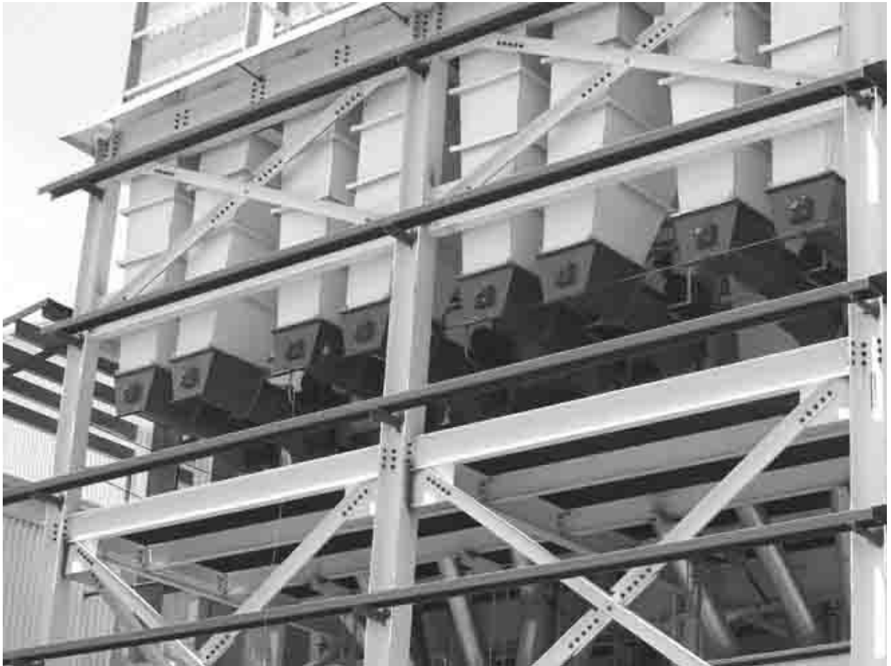
Screw Conveyors are performing their assigned tasks in virtually all types of industries and, in addition, special designs are being developed for use as components in machinery and equipment.
